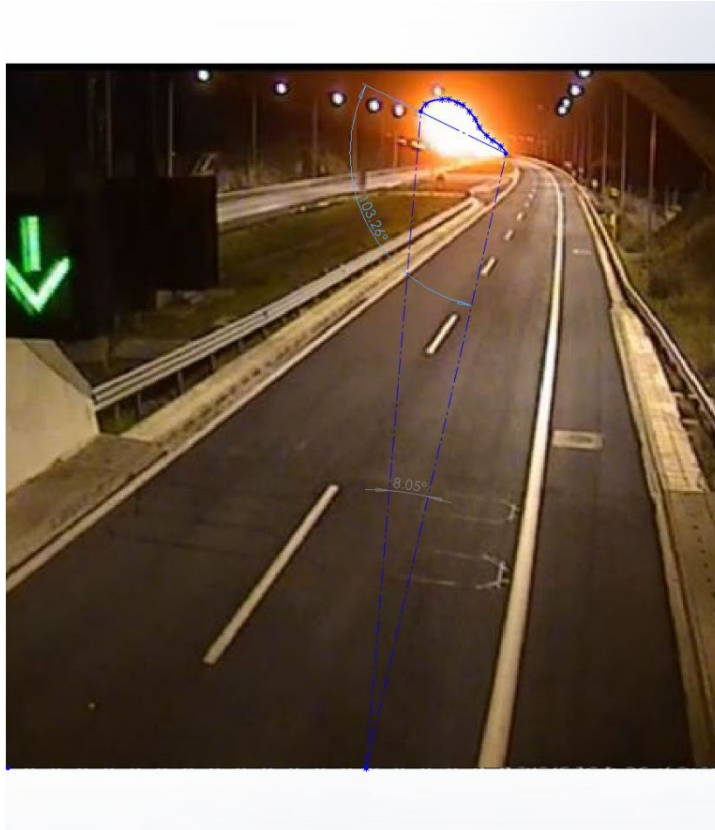
Figure 2. The triangle shows the calculation of the maximum length of the fireball. This is a frame extracted from one of the two videos in Exhibit A. The picture is extracted from Mr. Kokotsakis' report. The fireball maximum length as viewed from the Tempi 1 tunnel camera (located north of the accident site 750m away)
